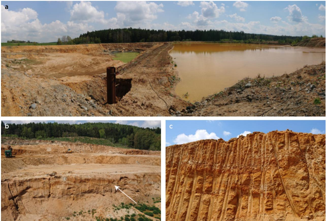
**Figure 4:** (a) The sand-and-gravel quarry near Chlum is expansive. The sediments lie on top of gneissic bedrock (exposed as the dark area on the far side of the smaller pit to the left). (b) Mining involves the use of excavators and trucks. A claystone horizon (indicated by the arrow) forms a darker brown layer in the pit wall in the foreground. (c) Moldavite is found in subhorizontal gravel layers. (The vertical lines are from the excavator used to mine the sediments.) Photos by T. Stephan.
