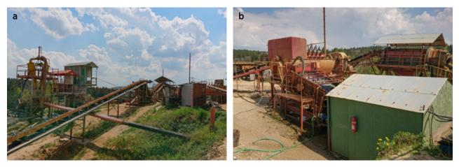
Figure 5: (a) The mined sediments are processed in this washing and sorting plant. (b) After screening out smaller size fractions, the moldavites are hand-picked in the green building. Photos by T. Stephan.
